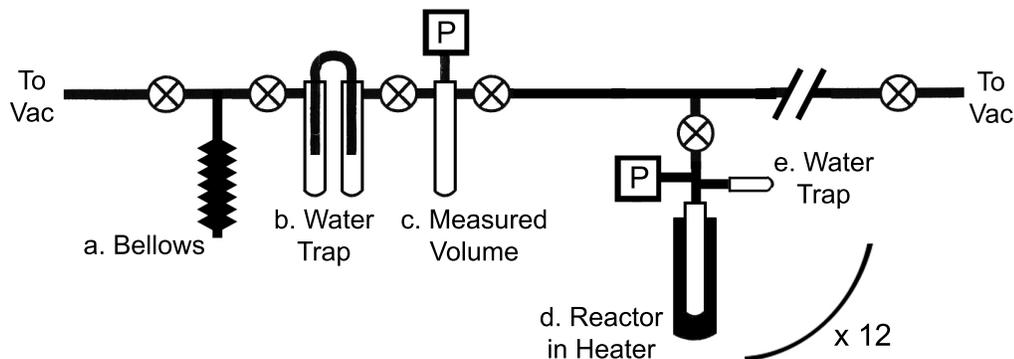
Figure 2.3: Schematic of the vacuum manifold used to transfer  $\text{CO}_2$  samples into individual reactors for graphitization at CAMS. The vacuum manifold contains 12 reactors which are configured in the same manner as the reactor pictured here.
