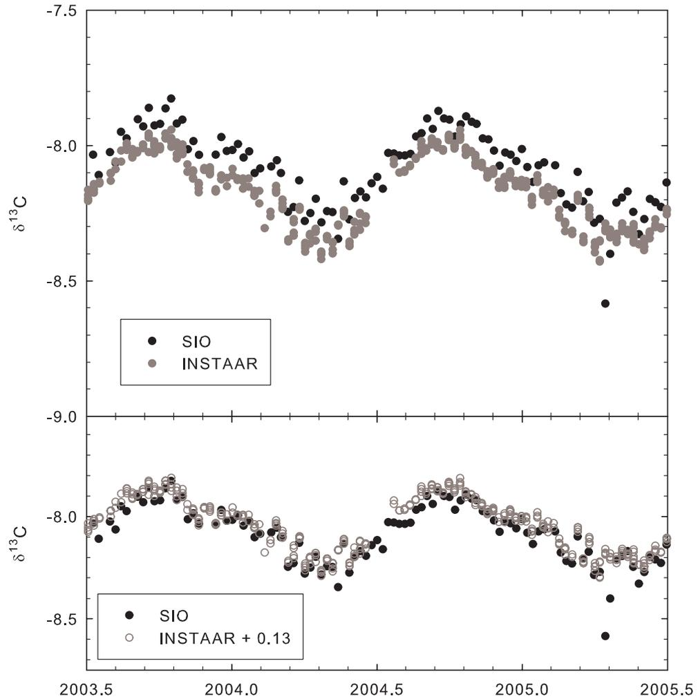
Figure 2.13: Scripps  $\delta^{13}\text{C}$  measurements at Mauna Loa and  $\delta^{13}\text{C}$  in  $\text{CO}_2$  measured at INSTAAR. The bottom panel includes an addition of 0.13 ‰ to the INSTAAR data.
