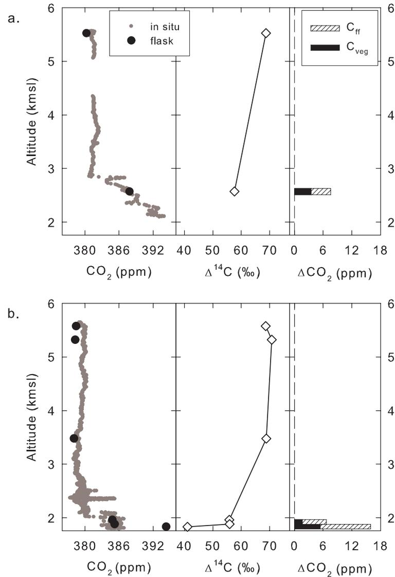
Figure 5.4: Profiles near 10 a.m. sampled in the urban area on a. May 20, 2004 and b. July 20, 2004. Measured CO<sub>2</sub> concentration (flask data in black circles; *in situ* data in gray circles), Δ<sup>14</sup>C (diamonds), and the amount of CO<sub>2</sub> added (ΔCO<sub>2</sub>) as C<sub>veg</sub> (black bars) and C<sub>ff</sub> (hatched bars). Altitude is given in km ASL, where the ground level is at the base of the plot (1.76 km ASL).
