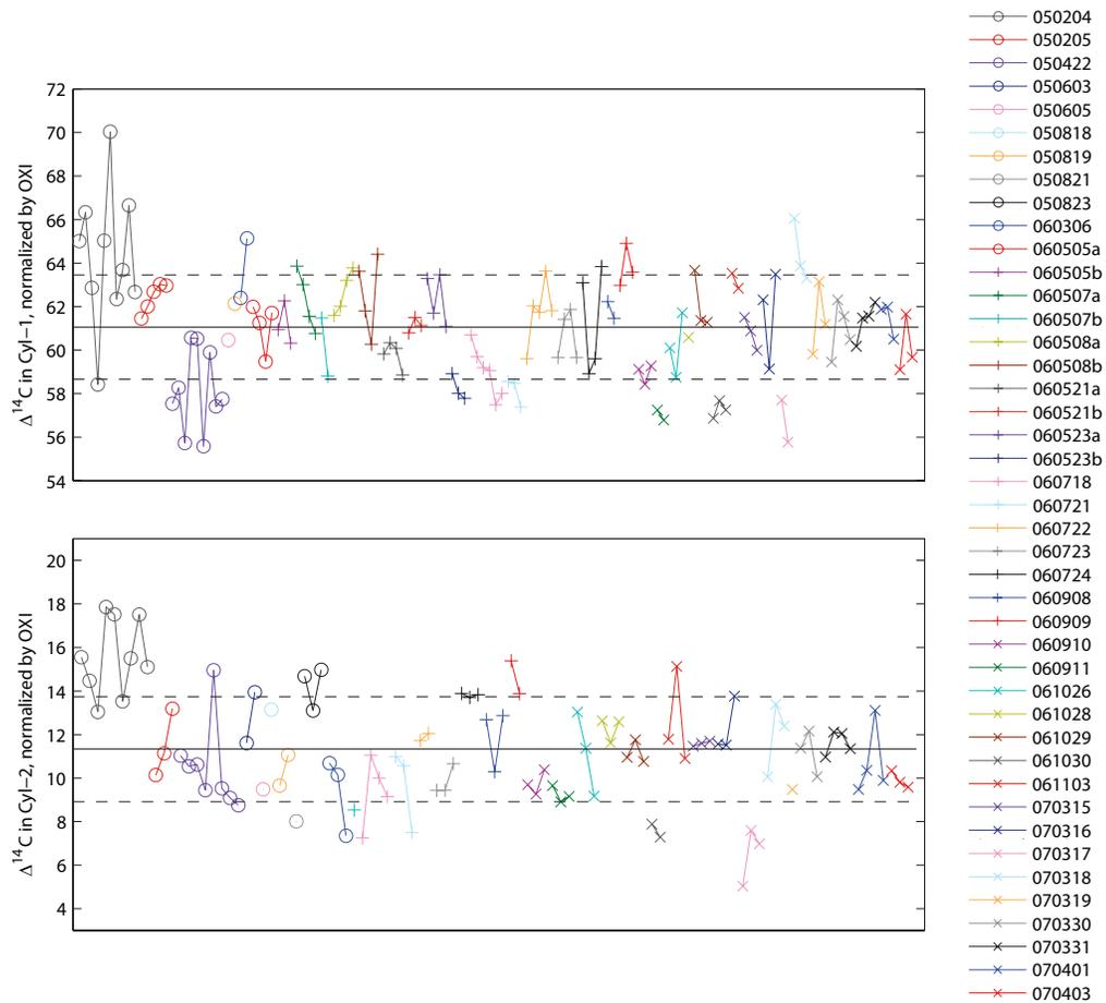
Figure 2.7: Measured  $\Delta^{14}\text{C}$  in Cyl-1 and Cyl-2, as normalized by OXI. Targets from different wheels are shown as different symbols; targets from each wheel are connected by straight lines. The solid line shows the mean values and the dashed lines show the overall standard deviation,  $61.0 \pm 2.4 \text{ ‰}$  for Cyl-1 and  $11.3 \pm 2.4 \text{ ‰}$  for Cyl-2.
