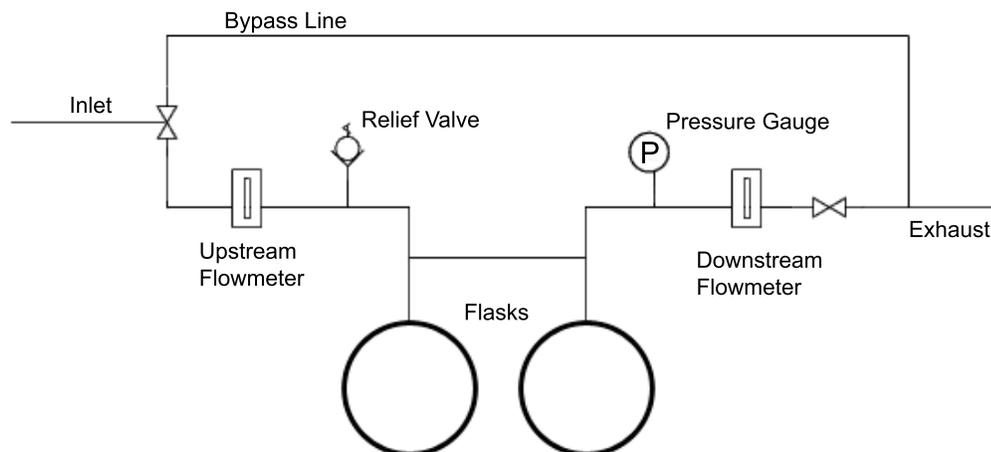
Figure 5.1: Schematic of the airborne flask sampling apparatus used in the ACME campaign
