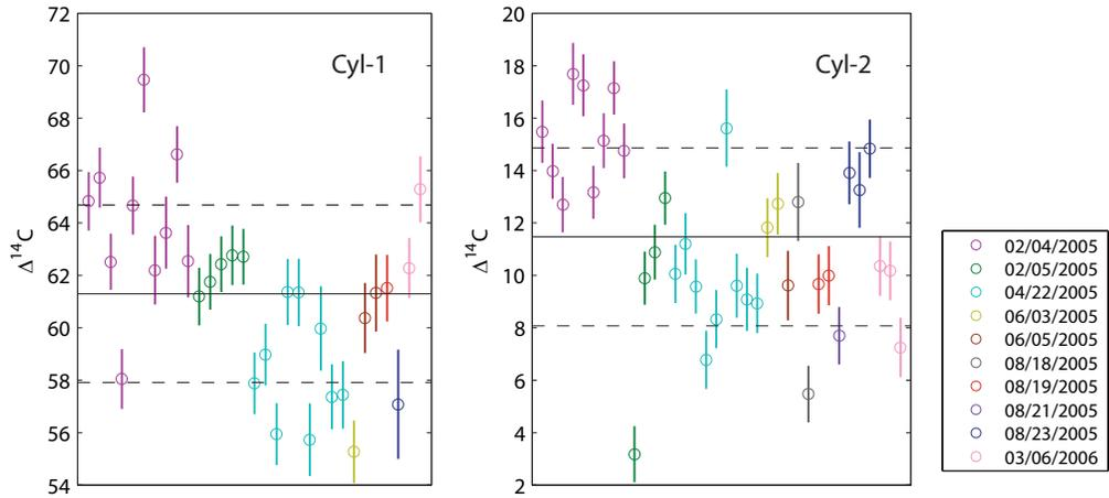
Figure 2.5: Measured  $\Delta^{14}\text{C}$  in Cyl-1 and Cyl-2 during analyses conducted over 9 wheels in 2005 and one wheel in 2006. Error bars show  $\sigma_{Int}$ , as calculated by 2.11. The solid line shows mean  $\Delta^{14}\text{C}$  and the dashed lines show 1-sigma deviation from the mean,  $61.3 \pm 3.4 \text{ ‰}$  for Cyl-1 and  $11.5 \pm 3.4 \text{ ‰}$  for Cyl-2.
