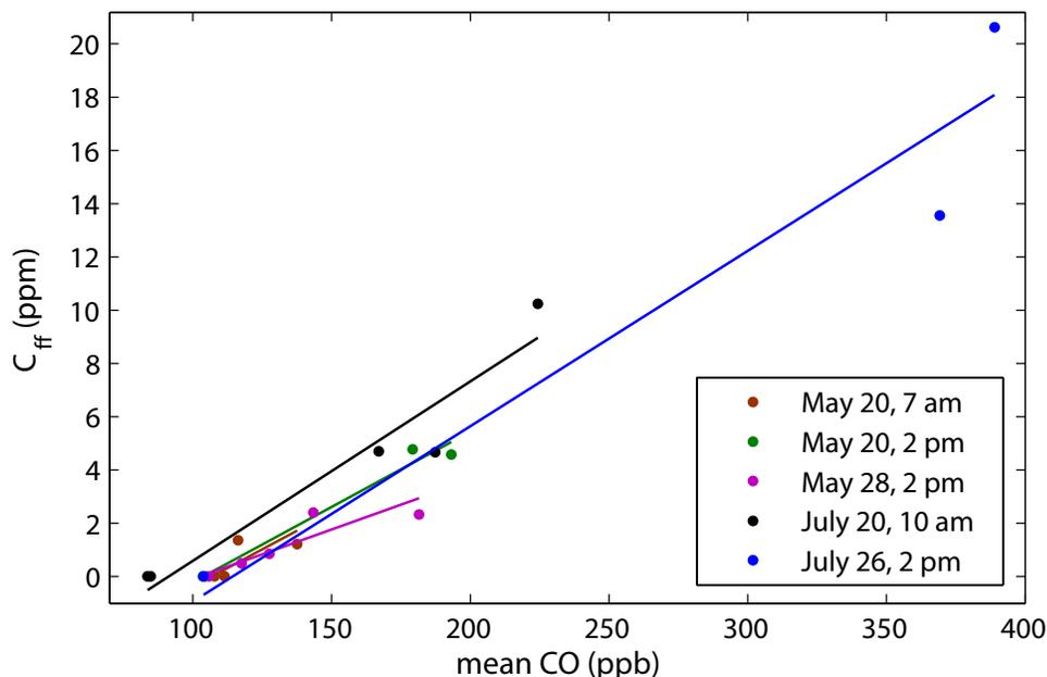
Figure 5.7:  $C_{ff}$  versus mean CO concentration measured *in situ* during the  $\sim 30$  second period during which the corresponding flask was sampled.  $C_{ff}$  and CO pairs are shown for 5 vertical profiles: May 20, 2004, 7 am (brown), May 20, 2004, 2 pm (green), May 28, 2004, 2 pm (purple), July 20, 2004, 10 am (black) and July 26, 2004, 7 am (blue). The lines resulting from geometric mean regressions on the  $C_{ff}$  and CO pairs are shown in corresponding colors.
