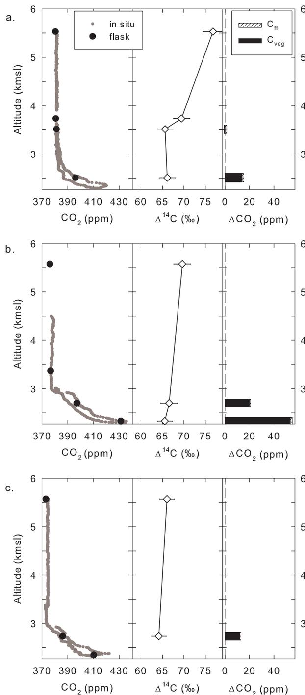
Figure 5.3: Profiles sampled near 7 a.m. in the rural area on a. May 20, 2004, b. July 22, 2004 and c. July 26, 2004. Measured CO<sub>2</sub> concentration (flask data in black circles; *in situ* data in gray circles), Δ<sup>14</sup>C (diamonds), and the amount of CO<sub>2</sub> added (ΔCO<sub>2</sub>) as C<sub>veg</sub> (black bars) and C<sub>ff</sub> (hatched bars). Altitude is given in km ASL, where the ground level is at the base of the plot (2.27 km ASL).
