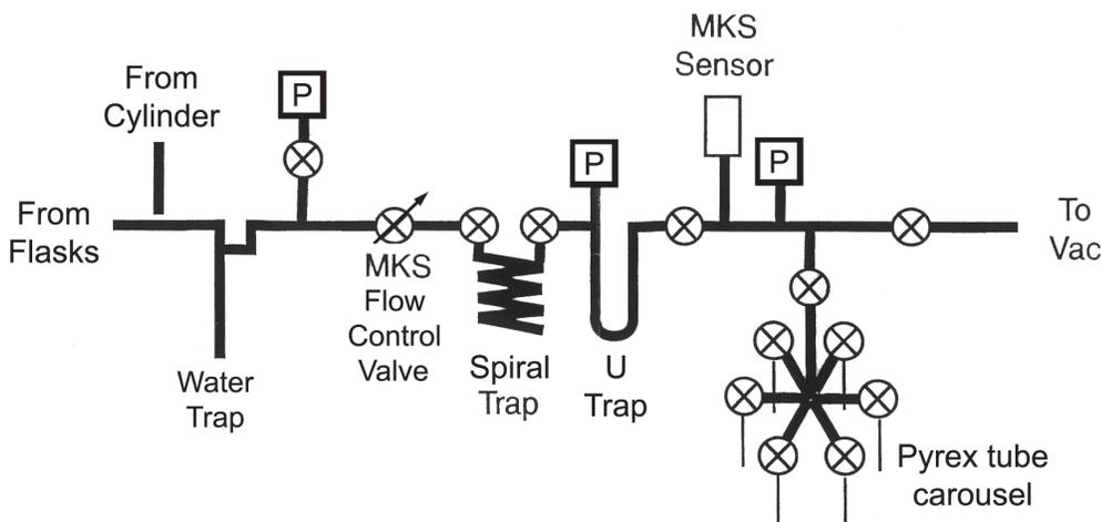
Figure 2.2: Schematic of the vacuum manifold used to perform CO<sub>2</sub> extractions from whole air flask samples and from whole air reference cylinders at Scripps.
