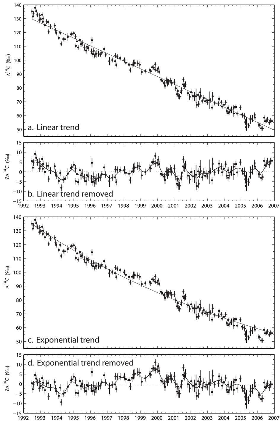
Figure 3.6:  $\Delta^{14}\text{C}$  observations from La Jolla fit to linear and exponential models (solid curves in a. and c., respectively). Residual  $\Delta^{14}\text{C}$  after subtraction of linear and exponential fits are shown in b. and d., respectively, where the solid curves show cubic smoothing splines through the residuals.
