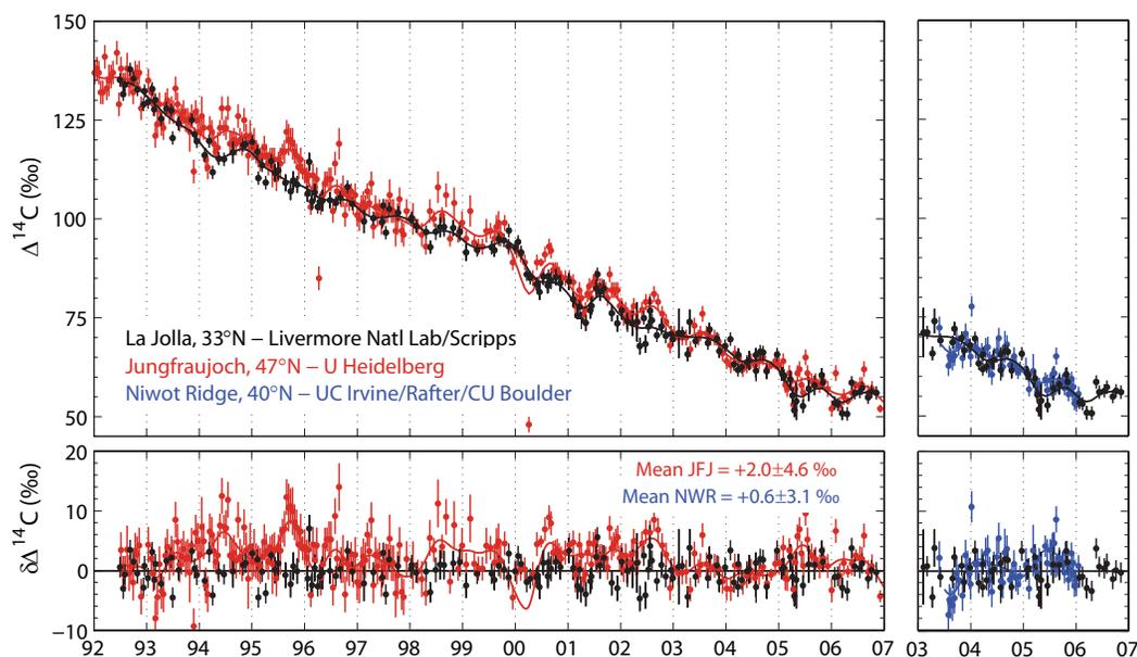
Figure 3.4: Comparison of  $\Delta^{14}\text{C}$  measured at La Jolla (black), Jungfraujoch (red, left) and Niwot Ridge (blue, right). The upper panels show measured  $\Delta^{14}\text{C}$  with uncertainties expressed as error bars and lines showing cubic smoothing spline curves fit to each time series. The lower panels show the difference from the smooth curve fit to measurements from La Jolla (black line in upper panels).
