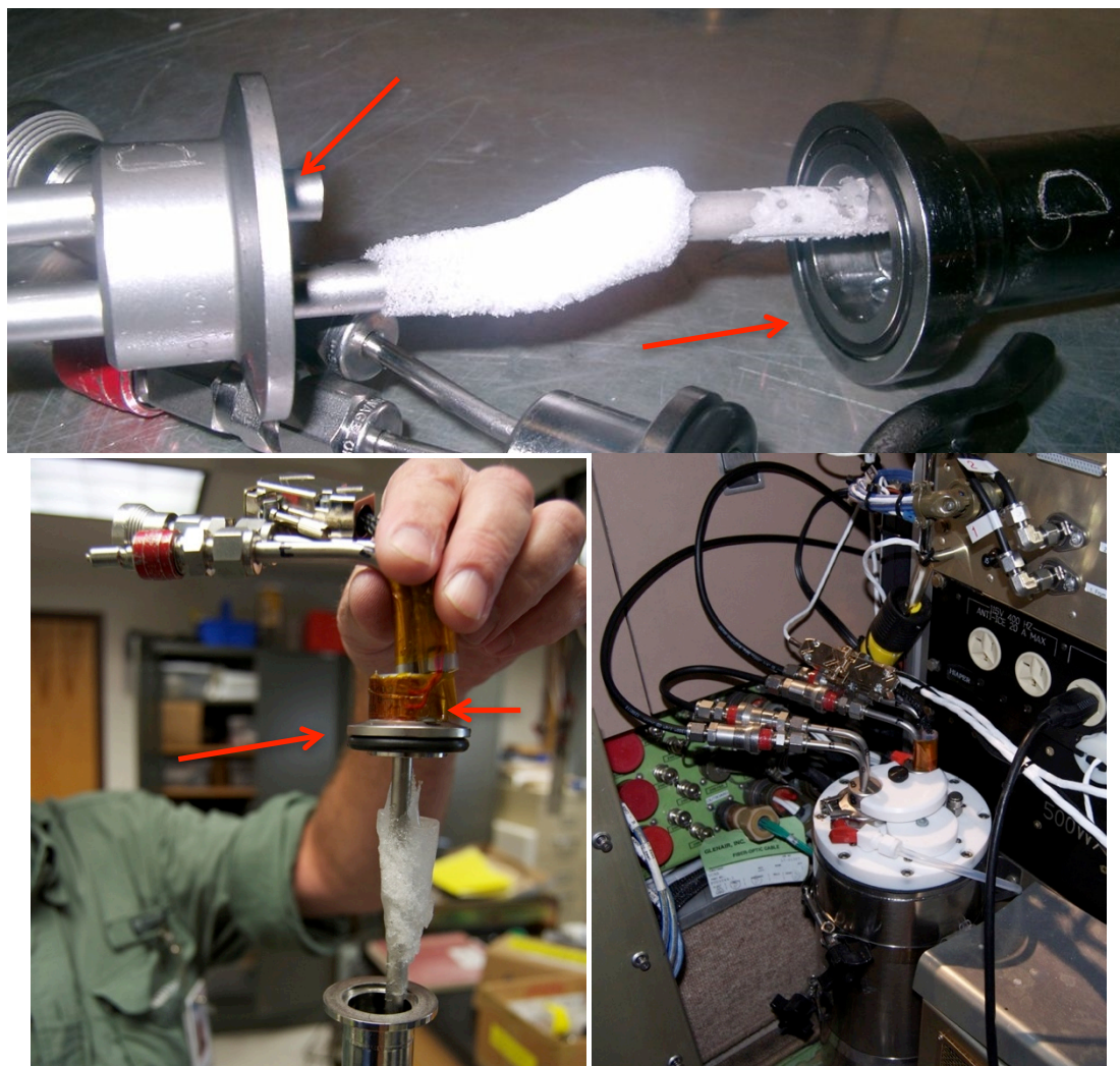
Figure 2.7. TOP: First generation MEDUSA trap design, showing small, custom inset O-ring groove and O-ring (right hand side) and unheated stainless steel inlet line (top left). BOTTOM LEFT: Second generation MEDUSA trap showing thicker O-ring. Shown is the upstream trap, which is equipped with a small surface heater (pointed to), seen encased in orange insulating tape near the top of the image. This maintains a non-freezing temperature at the short inlet diptube (obscured behind the longer out diptube) to prevent this area from freezing and stopping system flow. Both changes were instituted between HIPPO1 and HIPPO2. BOTTOM RIGHT: Second generation cryotrap installed in MEDUSA dewar. Sample air enters the upstream trap at the right from the pump box (not shown), circulates through the first trap and continues via a jumper to the downstream cryotrap at the left, and finally returns to the pump box.
